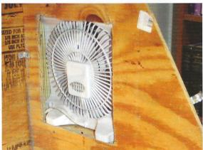
The smallest furnace filter available draws out paint particles; when it's dirty, it can be flipped over to use the other half.
